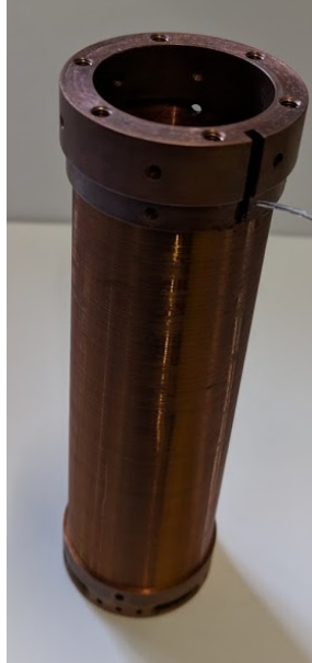
Figure 3.16: Image of the NMR Solenoid.
