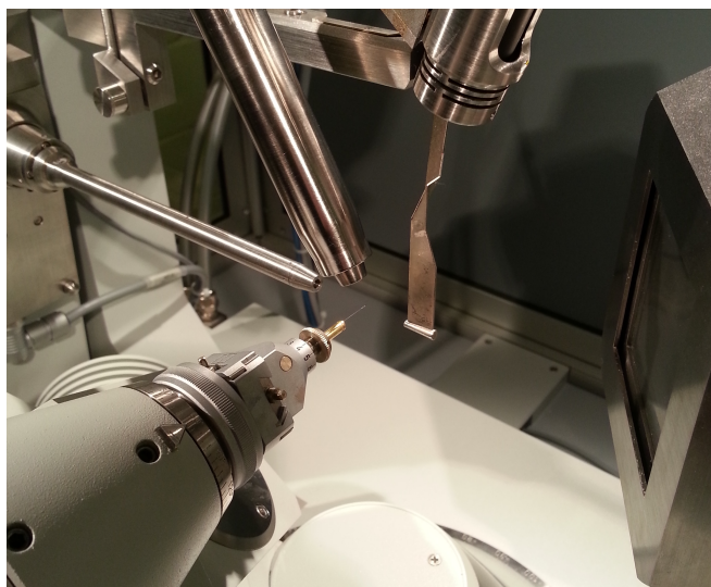
Figure 3.9: Xcalibur single crystal diffractometer at Royal Holloway
