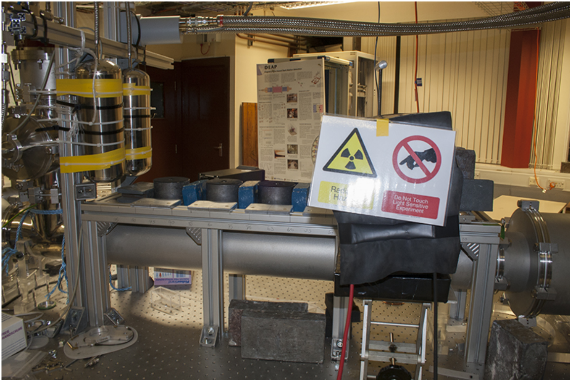
Figure 5.8: An image of the collimator set up for the argon fill 2. This collimators and lead shielding were moved every five runs to get data at different positions. The tag pmt is enclosed within the mobile dark box. The mobile dark box is shown on the right hand side, propped up and with a radiation safety sign attached.
