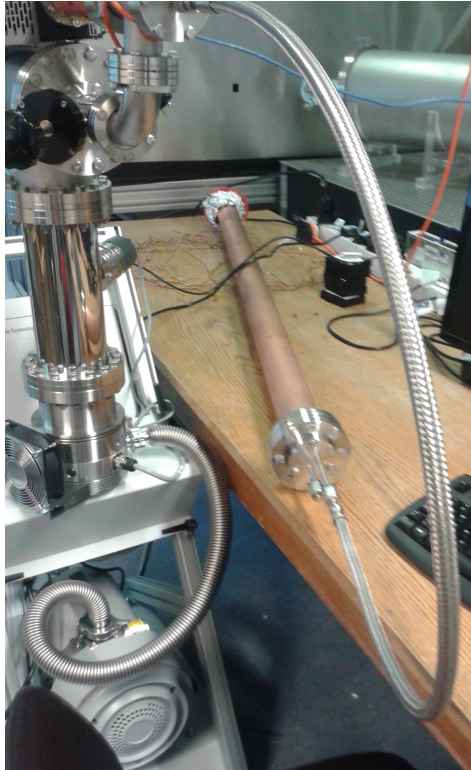
Figure 4.2: An image of the inner vessel before it was installed in the outer vessel. It is attached to vacuum system.
