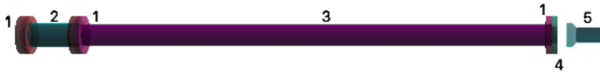
Figure 4.1: A visual representation of the simplest GEANT4 geometry model used to test the experimental concept. CF flanges(1), a stainless steel tube containing (2), a copper tube containing liquid argon (3), a TBP coated acrylic window coupled to a sapphire viewport (4), and a PMT (5).
