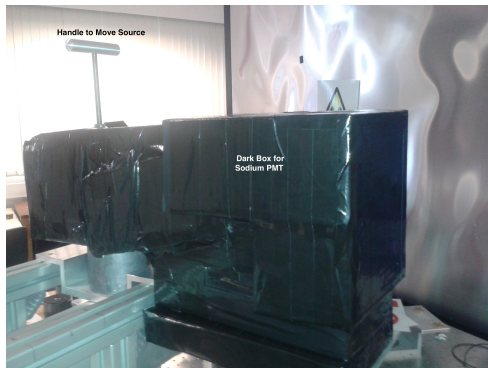
Figure 4.23: An image of the sodium PMT dark box. This was taken before the PMT was installed. Once the PMT was installed, the box was sealed to prevent light leaks.
