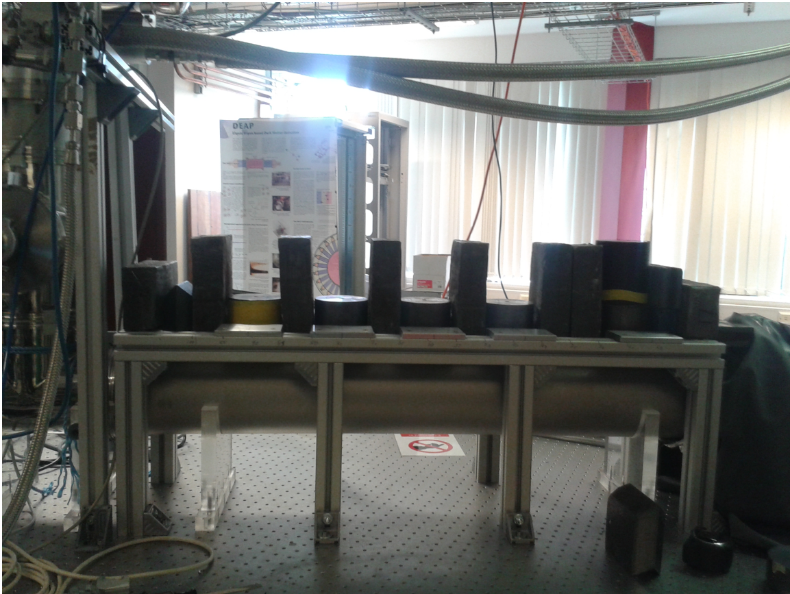
Figure 5.3: An image of the collimator set up for the argon fill 1. This collimators and lead shielding were moved every five runs to get data at different positions.
