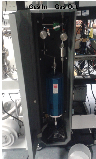
Figure 4.16: Image of the MonoTorr Heated gas getter used in the experiment.
