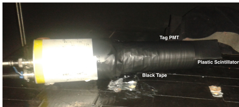
Figure 4.22: An image of the Sodium PMT. The plastic scintillator is coupled to the PMT window and this has all be wrapped in black tape.
