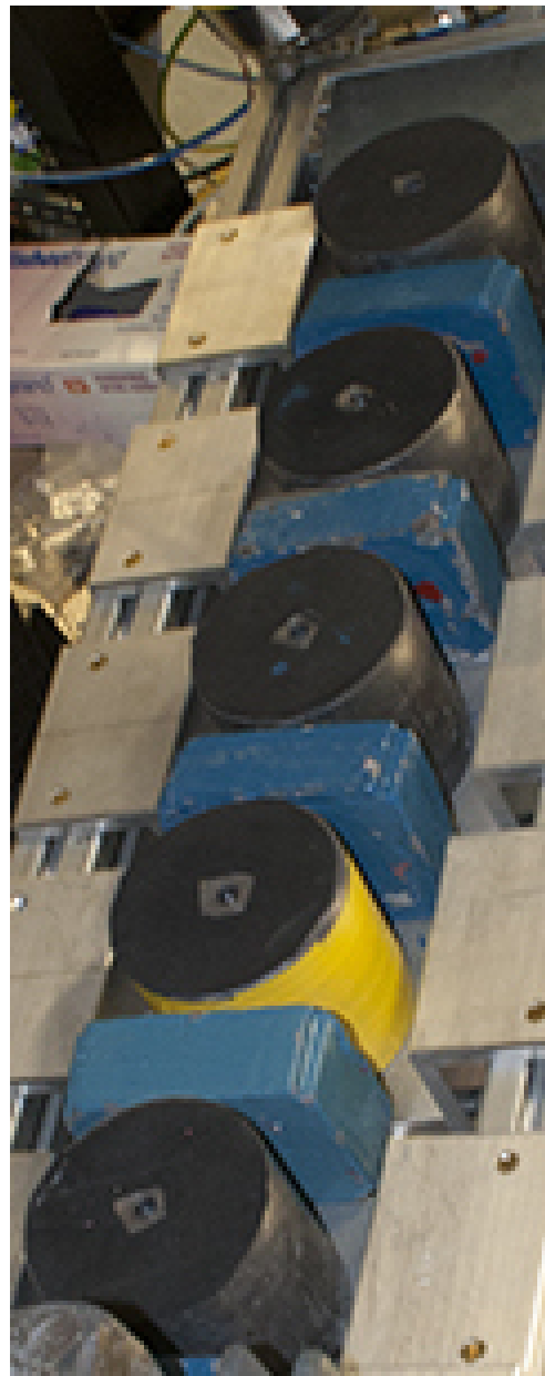
Figure 4.11: The collimators with black foam used for a light seal. Between each collimator is a lead block to reduce background from the source
