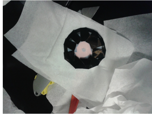
Figure 4.15: Spectral black folded around the front aperture to secure the TPB coated acrylic window.
