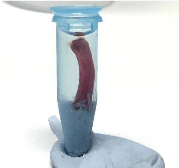
Figure 2.15: Scanning a large G1 using high resolution micro-CT. The G1 was placed inside a micro-centrifuge tube filled with 70% ethanol.
