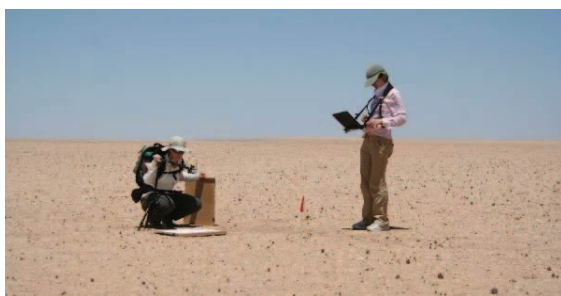
Figure 1: Measurements with the ASD spectrometer
