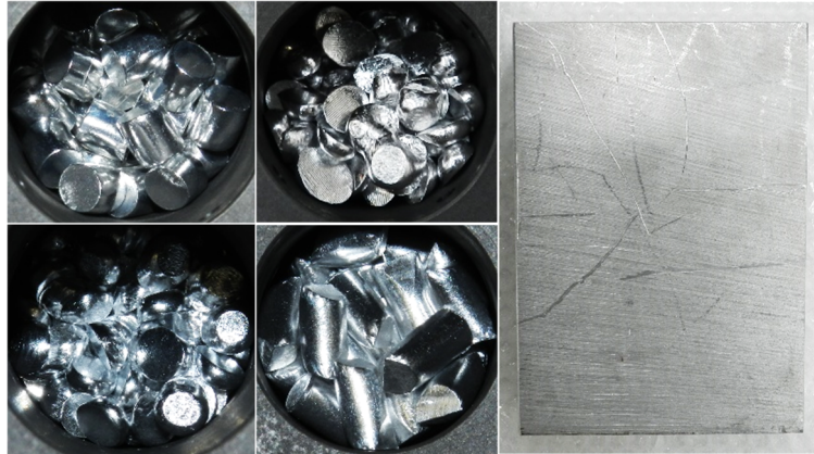
Figure 8: Metal samples supplied to this study: Alfa Aesar cylinders (top left), ESPI shots (top centre), Honeywell shots (bottom left), New Metals slugs (bottom centre) and the Sumitomo monolithic block (measuring 200 mm x 140 mm x 43 mm).
