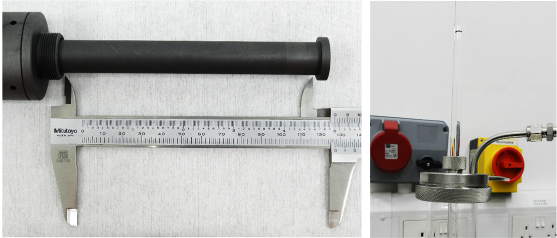
Figure 22: Measurement of the height of the re-entrant well to be pushed through the metal once it becomes liquid (left). Height transferred to the quartz rod to indicate when the insertion was complete.
