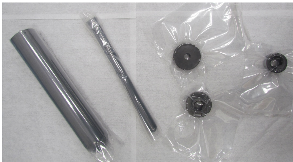
Figure 9: A set of specialty graphite components (SIGRAFINE R6300-P5, purity 99.999 5 %), supplied in vacuum sealed bags, selected and ready to be baked.
