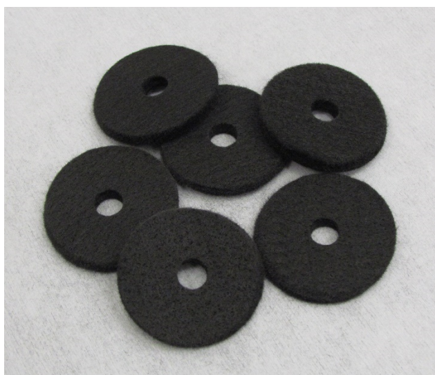
Figure 10: Graphite felt discs (SIGRATHERM® GFA5, purity 99.998 %) cut to fit the internal diameter of the quartz envelope, also allowing the insertion of quartz re-entrant tube.
