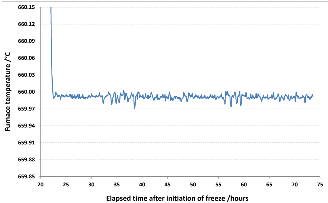
Figure 27: Set-point stability of furnace Fluke 9114 A63118 after freezing of cell Al-E (made from ESPI samples).
