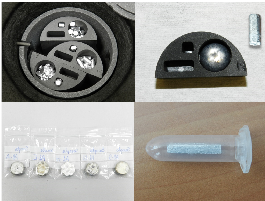
Figure 34: Preparation of the samples for GDMS analysis. Samples positioned in the furnace to be melted into the moulds (top left). Sample of aluminium supplied by New Metal made for NIM and NRC (top right). Collection of samples to be sent to NIM (bottom left). Pin after being cast and cut to the right size for NRC (bottom right).
