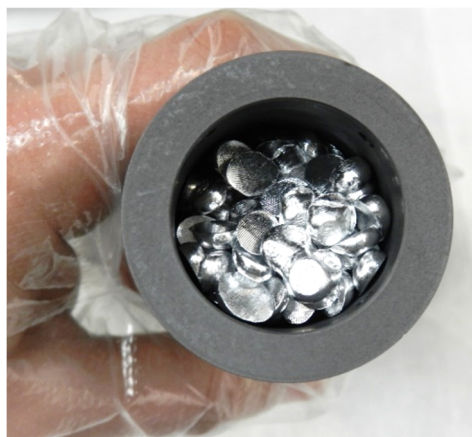
Figure 20: Crucible containing 200 g of aluminium shot, ready to be melted.
