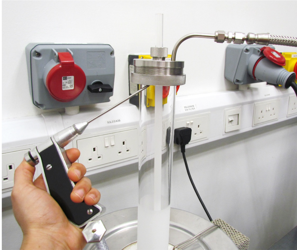
Figure 13: Testing the seals in the metal cap with the leak detector.
