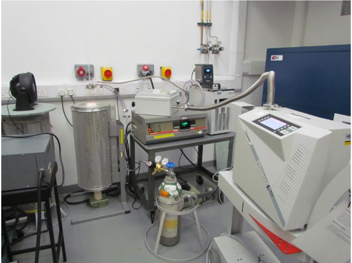
Figure 12: Set-up for the bake of the graphite pieces and casting of the ingots.
