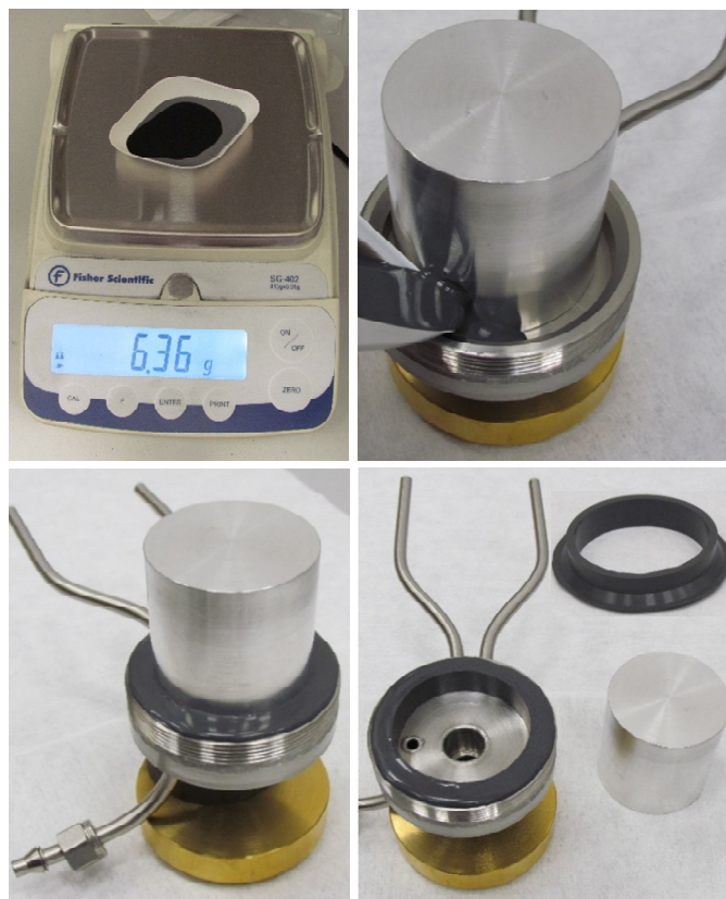
Figure 11: Highlights of the manufacture of the gasket made with two-part RTV silicone. From top-left: weighing and mixing the components; pouring the mixture into the mould; vulcanisation of the silicone and extraction of the gasket from the mould.
