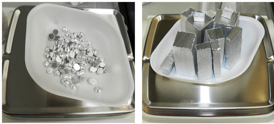
Figure 19: Weighing the portions of aluminium to transfer to the crucible. The first four cells were constructed with metal samples in the form of shot or slugs (left). The last cell (Al-S) was made using aluminium blocks cut from the larger sample sent by the supplier (right).
