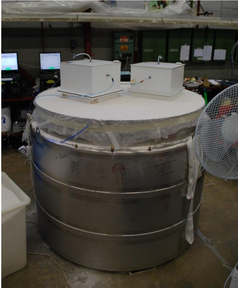
Figure 2.6: Calibration tank used for comparing N 2 O flux chambers at Hyttiala Forestry Research Station. Project funded by InGOS.
