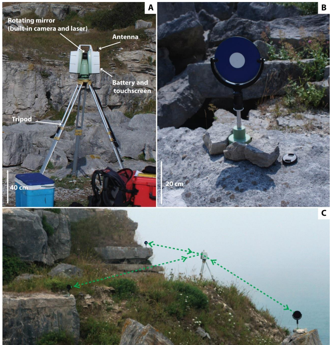
Figure 5.4 Lidar scanner characteristics. A – Details of the Leica ScanStation C10. B – Detail of one reflector used for the triangulation. C – Example of triangulation at Freshwater Bay.
