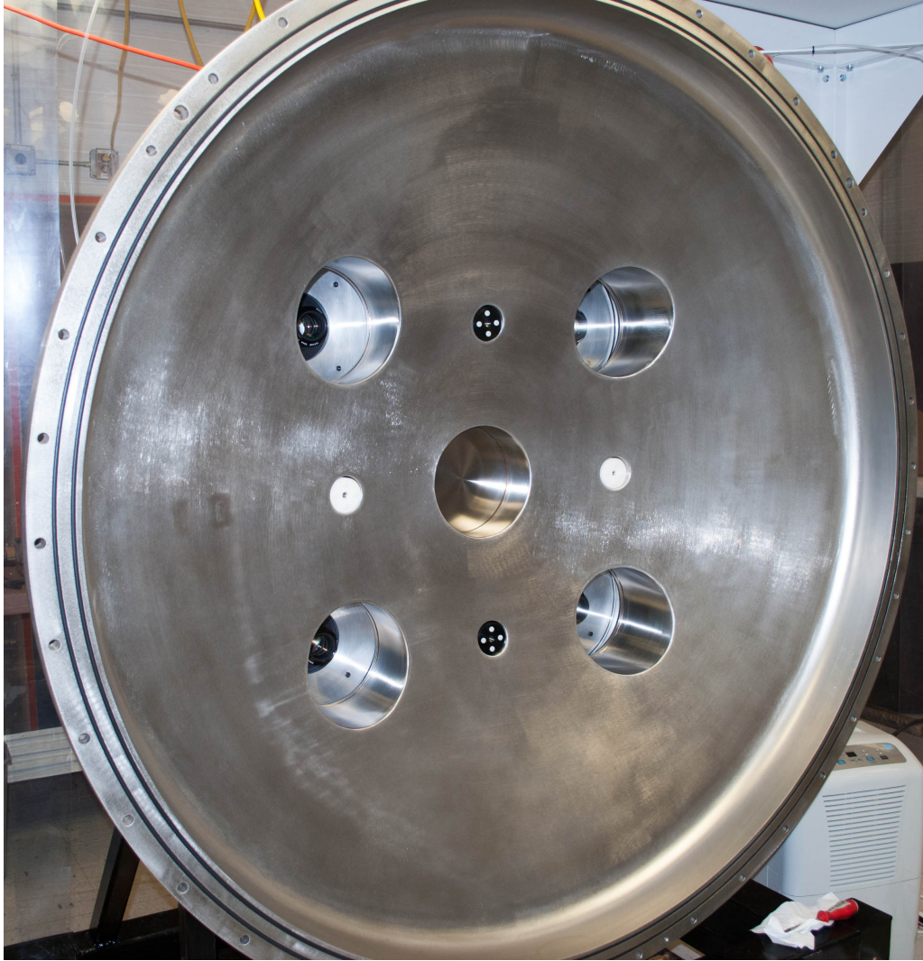
Figure 5-12: ^{55}\text{Fe} sources placed in the vacuum chamber door. The sources are the black and white circles located in-between the CCD windows.
