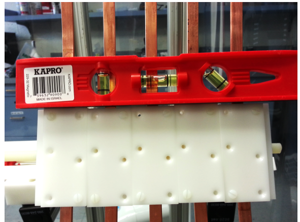
Figure 5-8: These pictures show the alignment of the field cage rings.
