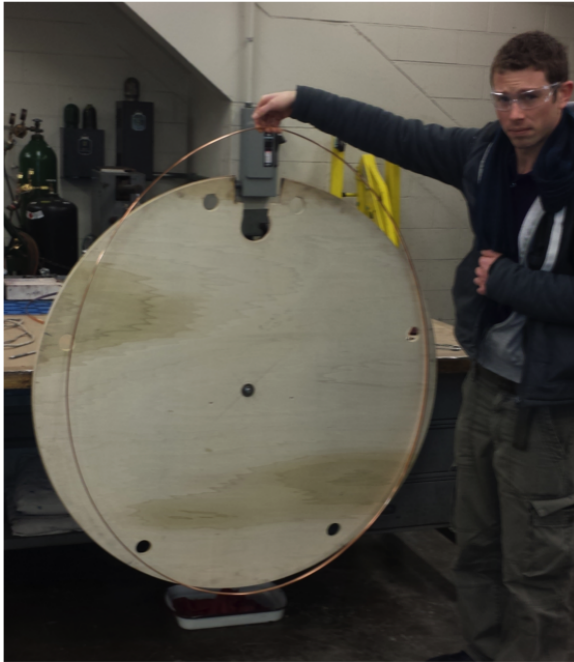
(a) Sagging of the soft copper ring.
