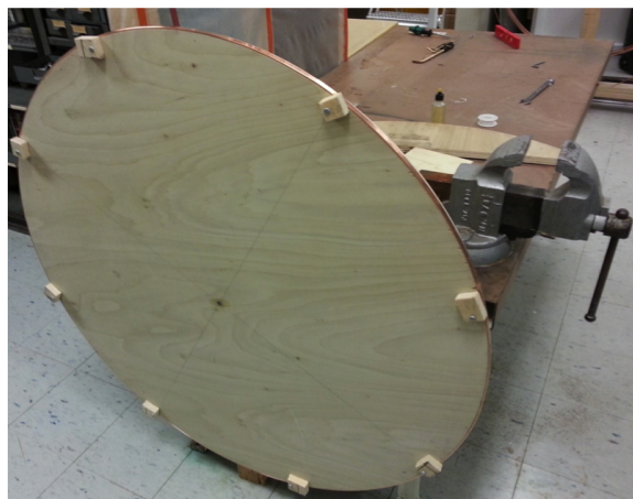
Figure 5-2: The frame used to harden the soft copper rings.
