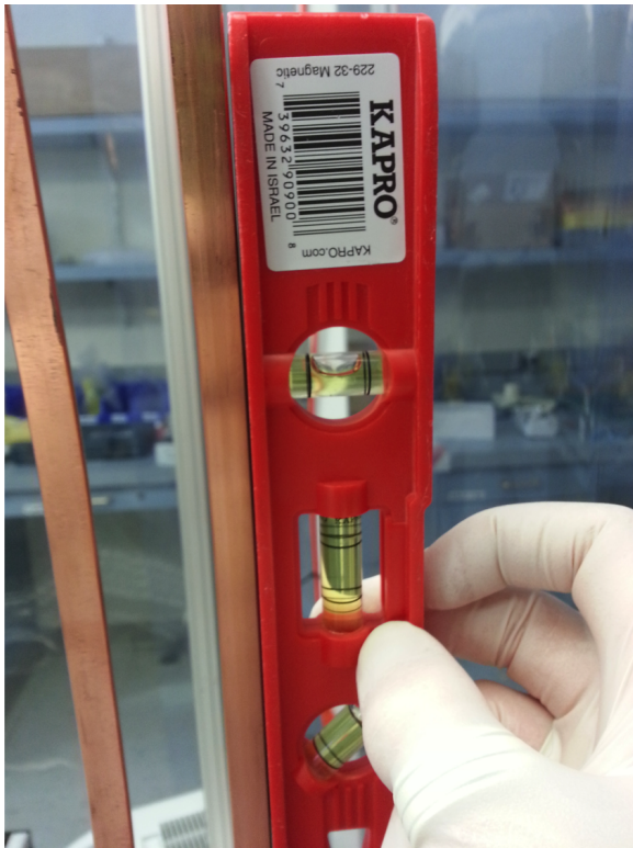
Figure 5-8: These pictures show the alignment of the field cage rings.
