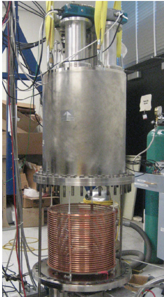
Figure 2-9: The 4Sh detector. In this image the TPC is exposed and can be identified by the copper structure in the lower section. The upper steel part is the bell-jar of the chamber and during operation sits over the top of the TPC, enclosing the volume.
