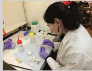
B. Cleaning procedure a) acetone & b) ethanol
