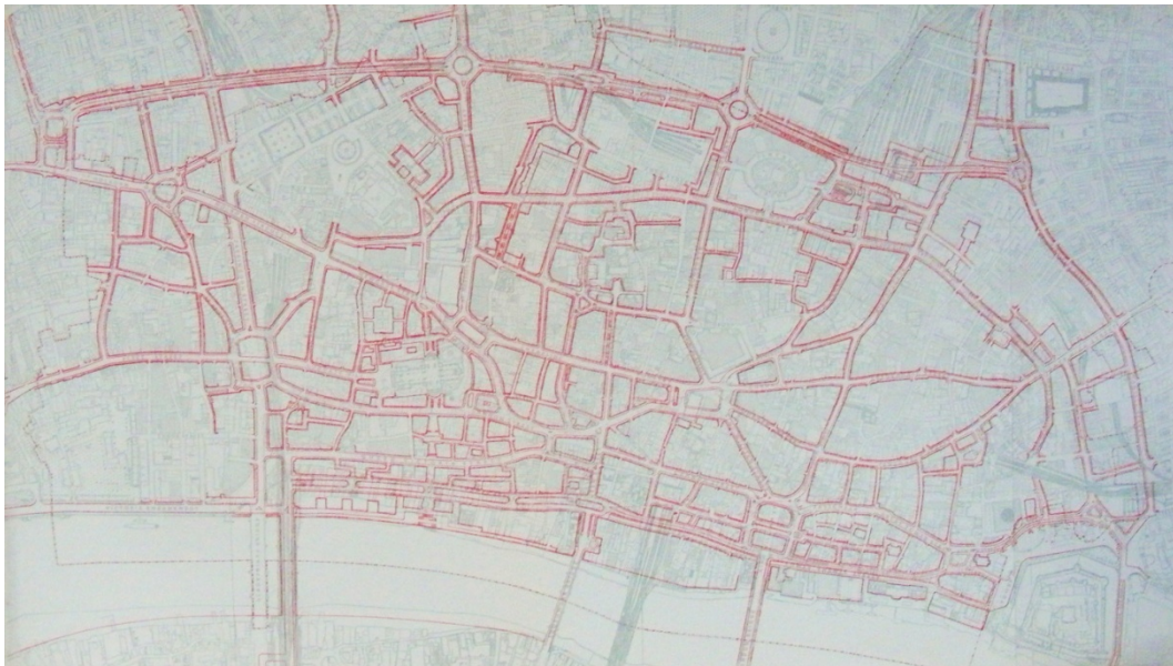
Figure 17: Proposed street plan for the City of London, 1947, showing new streets, building lines and pavements in red (Corporation of London, courtesy of London Metropolitan Archives). 182
