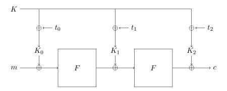
Figure 5.5: The 2-round EM scheme with a single permutation and a simple keyschedule
