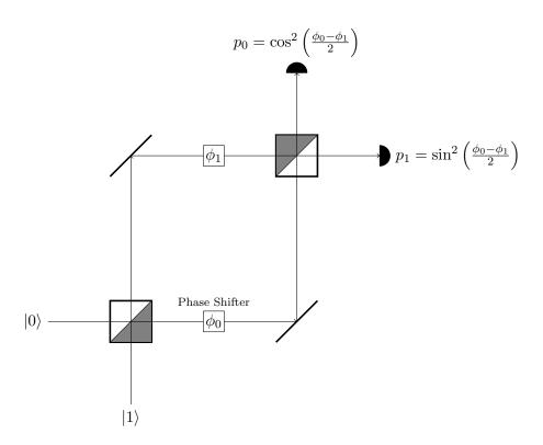
Figure 2.3: The Mach-Zehnder interferometer with two phase shifters. By adjusting the phase shifter, one can change the probabilities of photons striking the  $|1\rangle$  detector and the  $|0\rangle$  detector.
