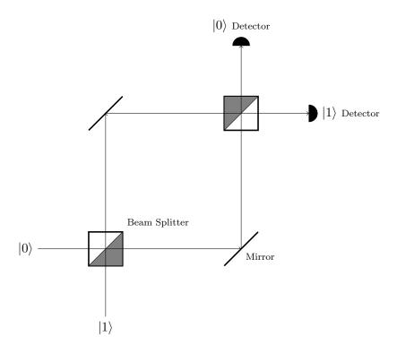
Figure 2.1: The Mach-Zehnder interferometer
