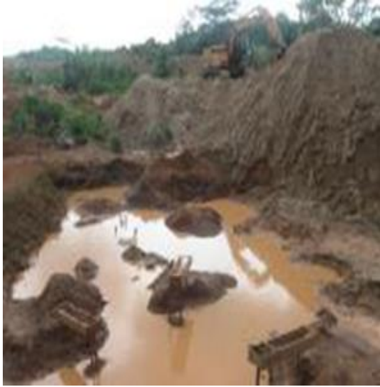
Open pit excavation of alluvial gold mining in Kambele III (Batouri)
