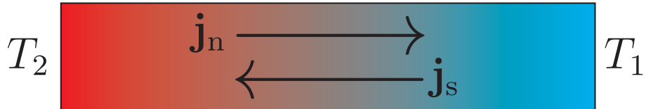
Figure 2.2: A rod of superconducting material with an established temperature gradient across its length is shown. The normal component of the current flows from one end of the rod to the other. Due to the requirement that the total current in a superconductor must be equal to zero the superconducting component flows in the opposite direction to compensate the normal current flow.
