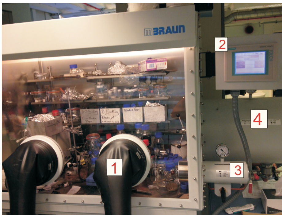
Figure 3.17: Photograph of one the MBraun glovebox that were used in this project. Various components are numbered; 1.) The 2 mm thick Viton ® gloves for handling 2.) Glovebox monitoring system 3.) Small port 4) Large port.
