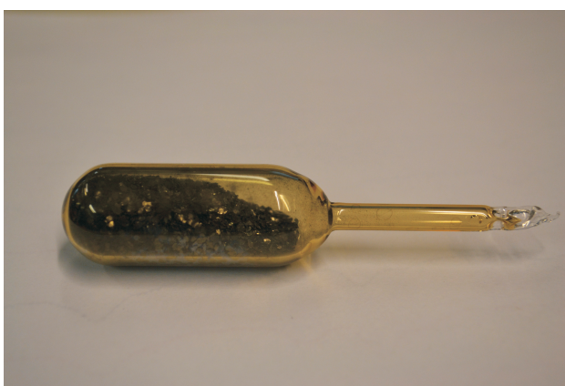
Figure 3.24: Pyrex ampoule that has been sealed with an oxy-acetylene torch, and then used to create a KC_y compound.
