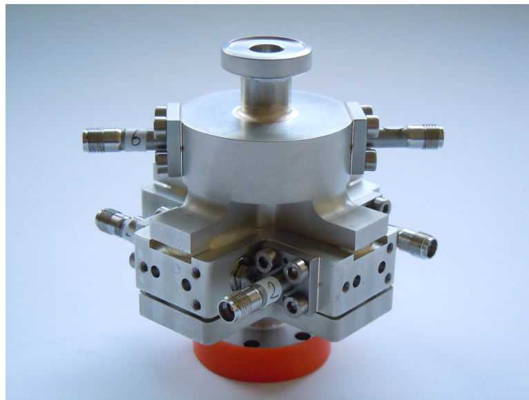
Figure 2.20: Image of the brazed cavity assembly.
