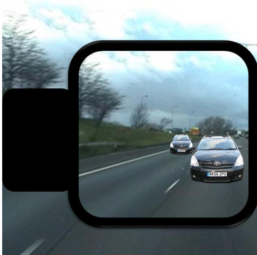
Figure 5.4: A simplified diagram of the driver mirror view when merging onto a high speed road. The driver needs to judge whether it is safe to merge in front of the car located in the nearside lane, but our experiments demonstrate that the greater optical size of the car in the adjacent lane may impact this judgement.
