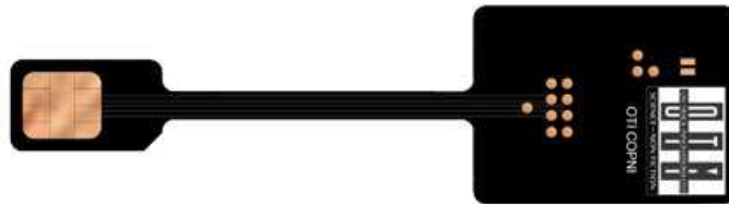
Figure 2.12: A SIM+antenna NFC solution by On Track Innovations (OTI) [31]
